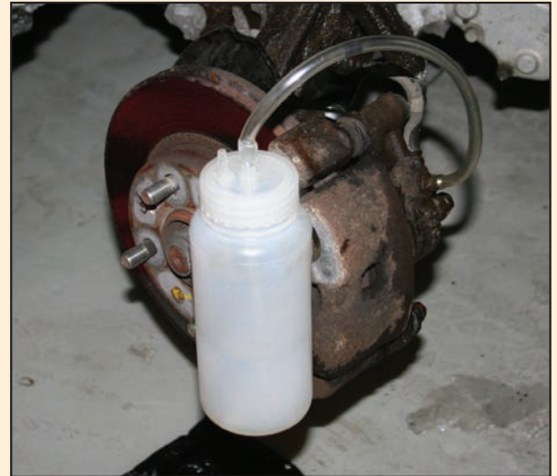
Waste Fluid Bottle connects to vehicle's bleeder screws
