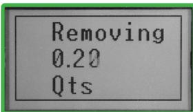
Check the fluid level. Press or to add or remove fluid in 2/10 of a quart increments. Use **option 3** in the main menu to add a full quart and **option 4** to remove a full quart.
