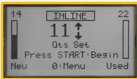
Use the arrow keys to select the desired amount to be exchanged. Press to proceed. Turn vehicle's **engine on**.
