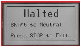
If the exchange stops and the display reads "Shift to Neutral", set the vehicle's parking brake, shift to Neutral, and press
