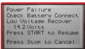
If there is a power failure during a transmission fluid exchange, the procedure can be continued seamlessly.
