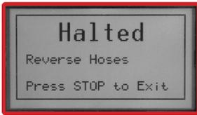
If the exchange stops and the display reads "Reverse Hoses", turn vehicle **off**, switch the red and black service hoses, restart vehicle, and press
