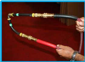
Make sure there is fluid in the New Fluid Tank. Connect the Red and Black service hoses together using any two mating adapters.
