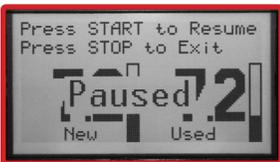
If needed, while running, pressing once will pause the machine. Press to resume from pause, or press a second time to cancel the exchange
