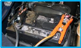
Connect battery cables to vehicle's battery.
