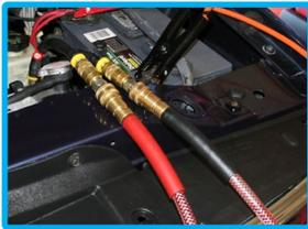
Connect appropriate adapters to vehicle's cooler line fittings.
