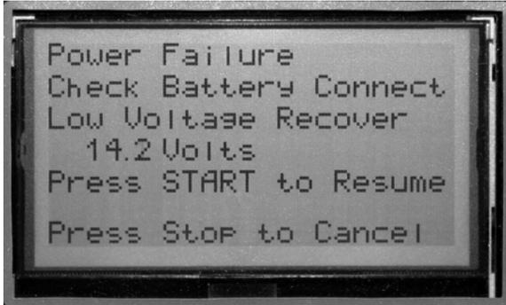
**Solution 1:** Check battery connection. Make sure there are no loose connections, and the machine's battery clips are not reversed. Remove all corrosion from the battery terminals. Make sure vehicle's A/C system is turned off.
